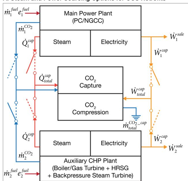
**B. Auxiliary CHP Plant with Boiler + BPT**
