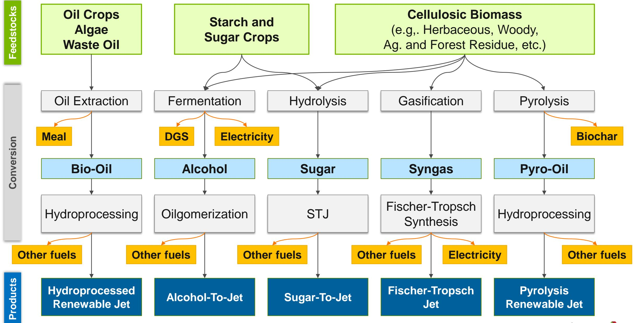
Note: DGS denotes Distillers' Grains with Solubles. Other fuels include fuel gas, naphtha and distillates
