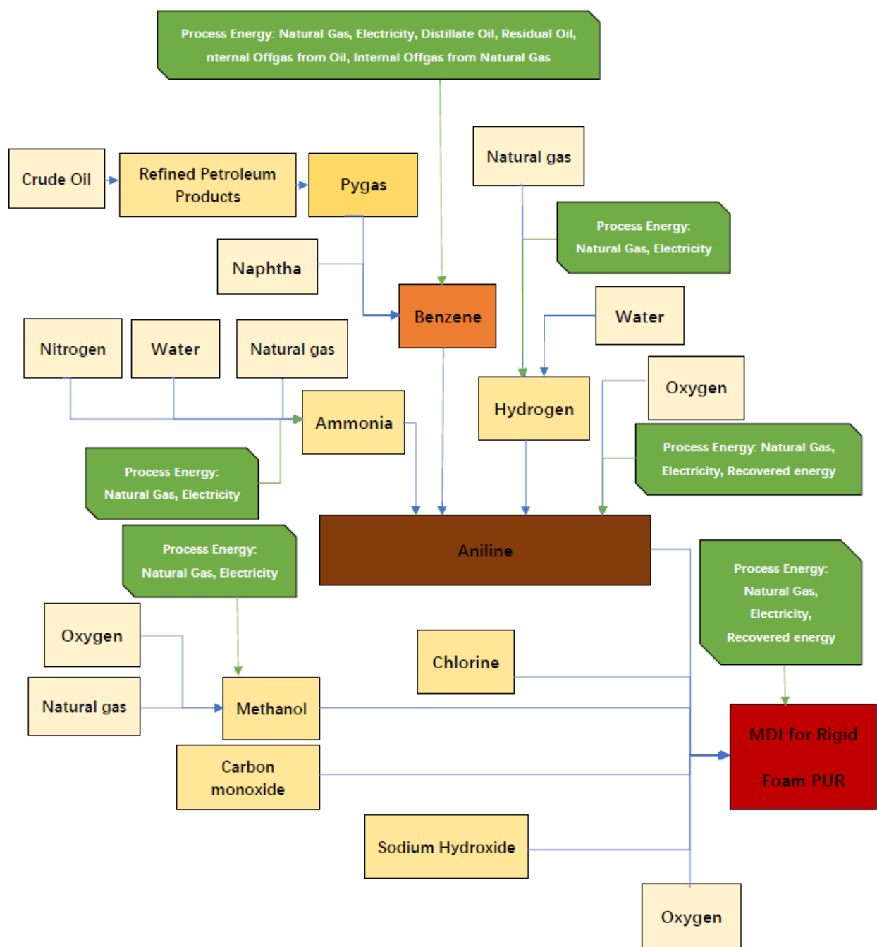
FIGURE A9. Manufacturing process of methylene diphenylene diisocyanate (MDI) as described in literature.
